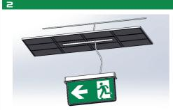
Connect the lead wire to the external lead wire of the sign (pay attention to the corresponding connection of live wire/neutral wire).
